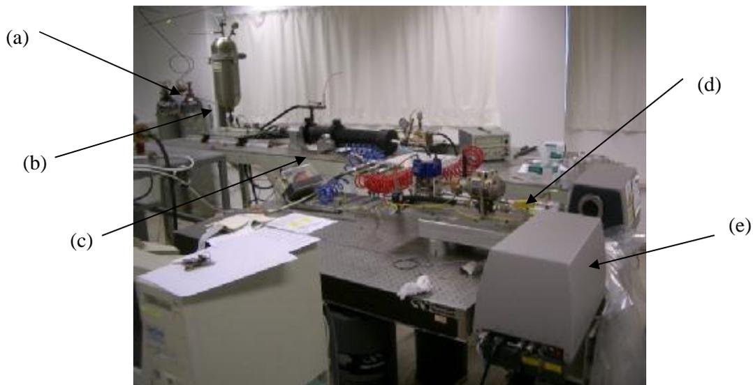
Figure 2. The experimental setup: (a) nitrogen tank for the nitrogen feed system, (b) hydraulic fluid pressure tank, (c) water/gel cylinder with piston, (d) atomizer head, (e) Malvern Mastersizer X.
